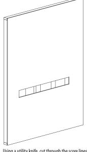
Using a utility knife, cut through the score lines and remove the 6" wide strip of drywall. The length of the opening should be equal to the length of the cabinets, PLUS the distance to the next wall stud in each direction.
