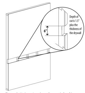
Place your  $2 \times 6$  in the opening and score a line across the face of the studs. Use a circular saw to make two cuts to the appropriate depth (1.5" deep on the stud, PLUS the thickness of the drywall); one on the pencil line and one on the bottom edge of drywall.
