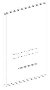
Cut ledge strip 2 inches less than run length. Center on run and fasten to studs usina 3" screws.
