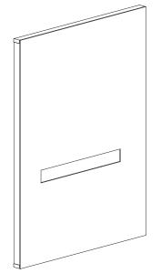
Place 2x6 in the notched area and secure with (2) 3"screws and construction adhesive on each stud. The face of the 2x6 should be flush with the surface of the studs.
